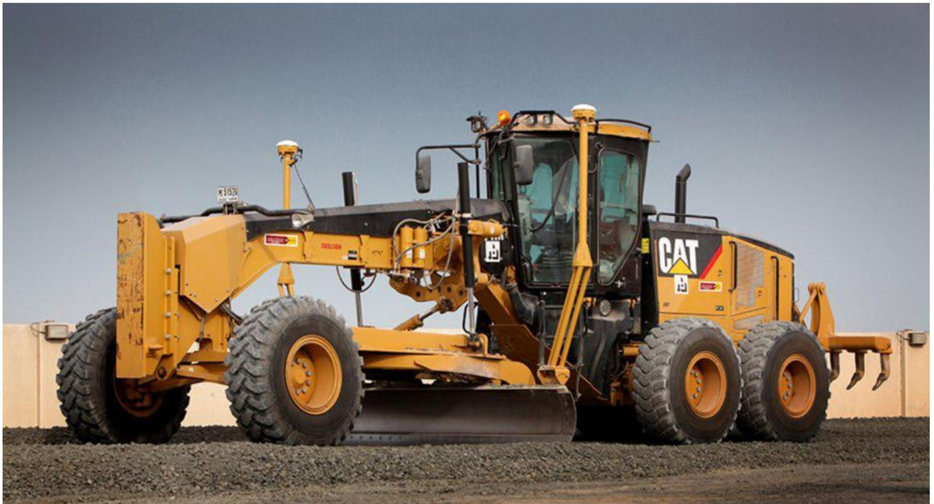
*Trimble GCS900 3D Grade Control System for Motor Grader.*
